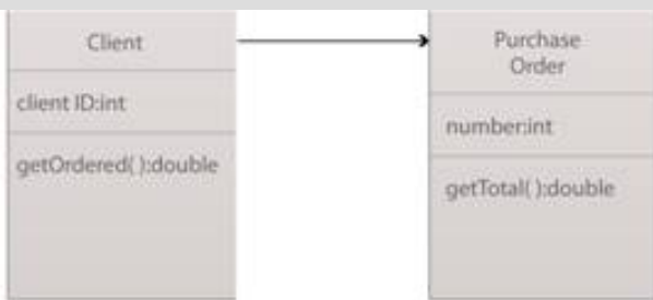
Figure 10: The Client class has an association with the Purchase Order class (top) similar to how the Client service relates to the Purchase Order service (bottom).
