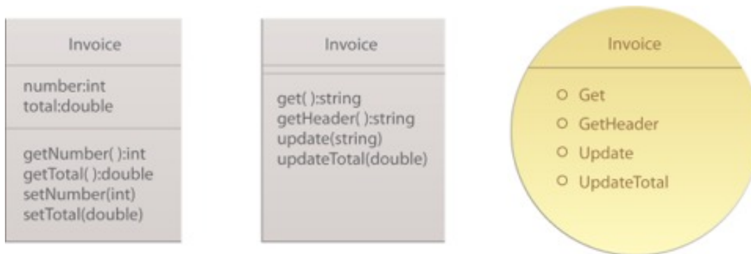
Figure 6: An object-oriented class (left), a service-oriented class (middle), and a service contract (right). Note that the attributes omitted by the middle class are public.
